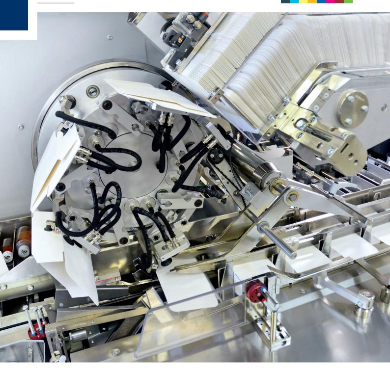
The operator side of the **HV** is perfectly linear and accessible, allowing carton magazine loading to be carried-out with convenience and with large carton storage capacity. This feature also gives the operator full vision and total control of all the functions carried-out on the machine.
