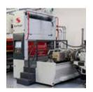
The optimized film take-off with nip roller and water suction for low and high denier tapes allows production speeds of up to 550 meters per minute.
