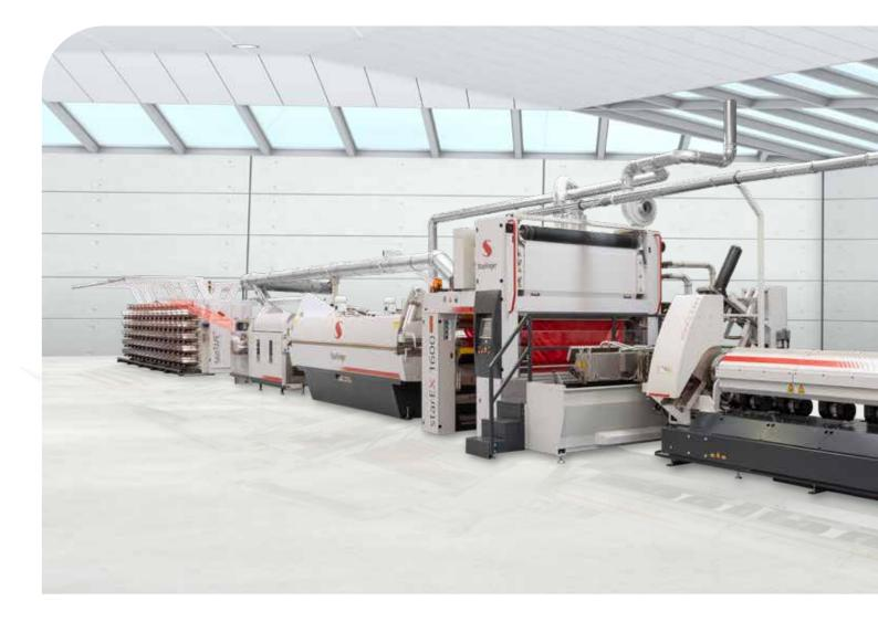
**The starEX 1600** is specially designed to extrude PP or HDPE/LLDPE tapes for high-performance applications at **premium quality** and **lowest cost**. The tapes are mainly used for producing woven bags, FIBC fabrics and in various other technical applications, in combination with a Starlinger piston filter system fabrics with high content of rPP or CaCO<sub>3</sub> can be produced.
