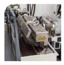
State-of-the-art extrusion unit with resource filter systems and high performance flat die. Energy-saving drive and machine design.
